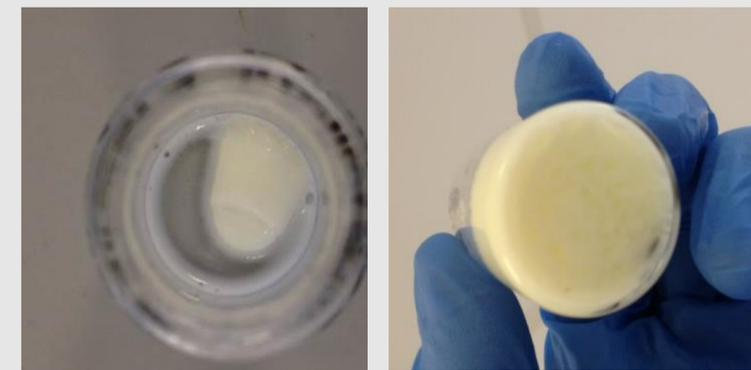
Figure 1: Capsules after 40minutes reconstitution in warm milk. Left, a gelatin capsule. Right, a pullulan capsule. A large remnant is visible with the gelatin capsule.
