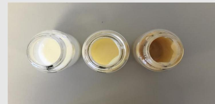
Figure 2: Reconstitution of Miglyol filled pullulan capsules in cold milk (left), custard (centre) and fruit puree (right).
